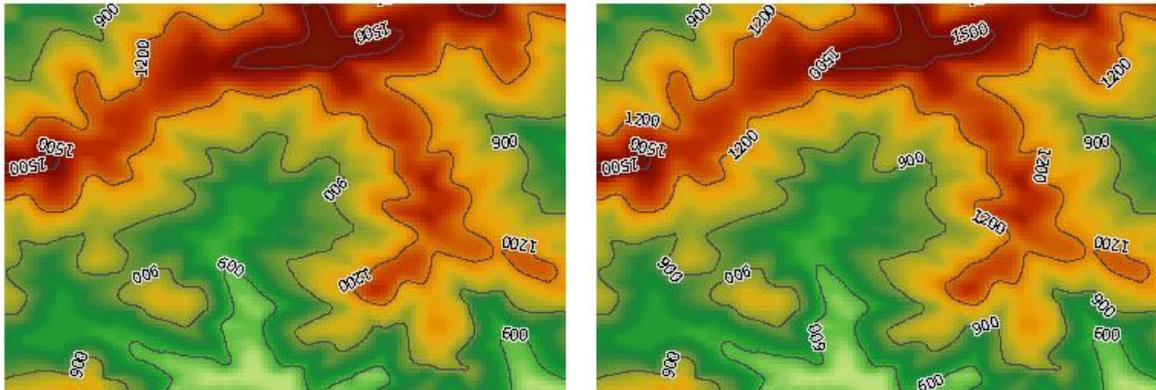
Remove Repeat Label is used to remove multiple repeat labels if a line object contains several subobjects. If Remove Repeat Label is unchecked, every subobject is labeled; if checked, only the maximum subobject within visual extent is labeled.
